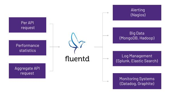
API requests, performance statistics, and license data are logged for review. The administration console provides aggregate analysis. For detailed data discovery MVIS communicates with Fluentd, which formats the logs for consumption by popular log management tools. Investigate issues that impact performance or end-user experience and determine if license redistribution or more licenses are needed.
